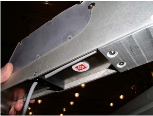
Figure 5. RFID tag on Hover-Davis tape feeder
