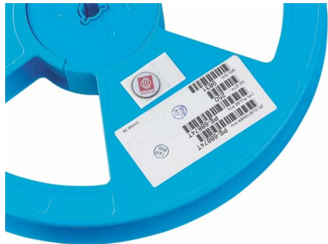
Figure 2. Re-usable RFID tag on Reel
