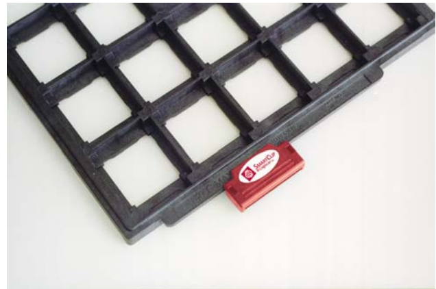
Figure 1. Re-usable RFID tag on JEDEC tray
