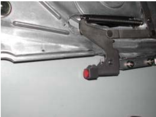
Figure 4. RFID tag on Juki tape feeder
